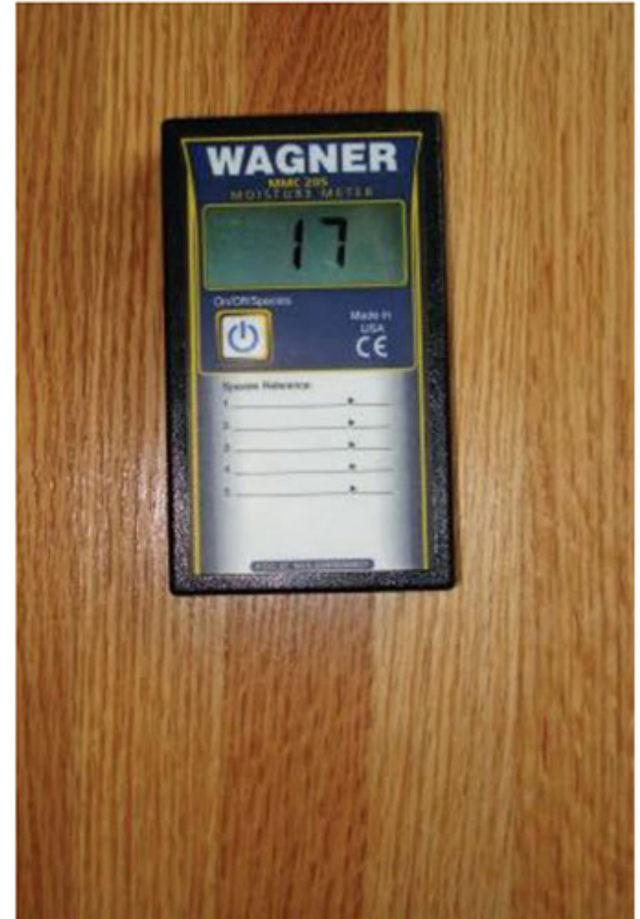
Before-and-after moisture readings should be taken. The above photos illustrate an eight-percent moisture gain, which is dangerously high.
