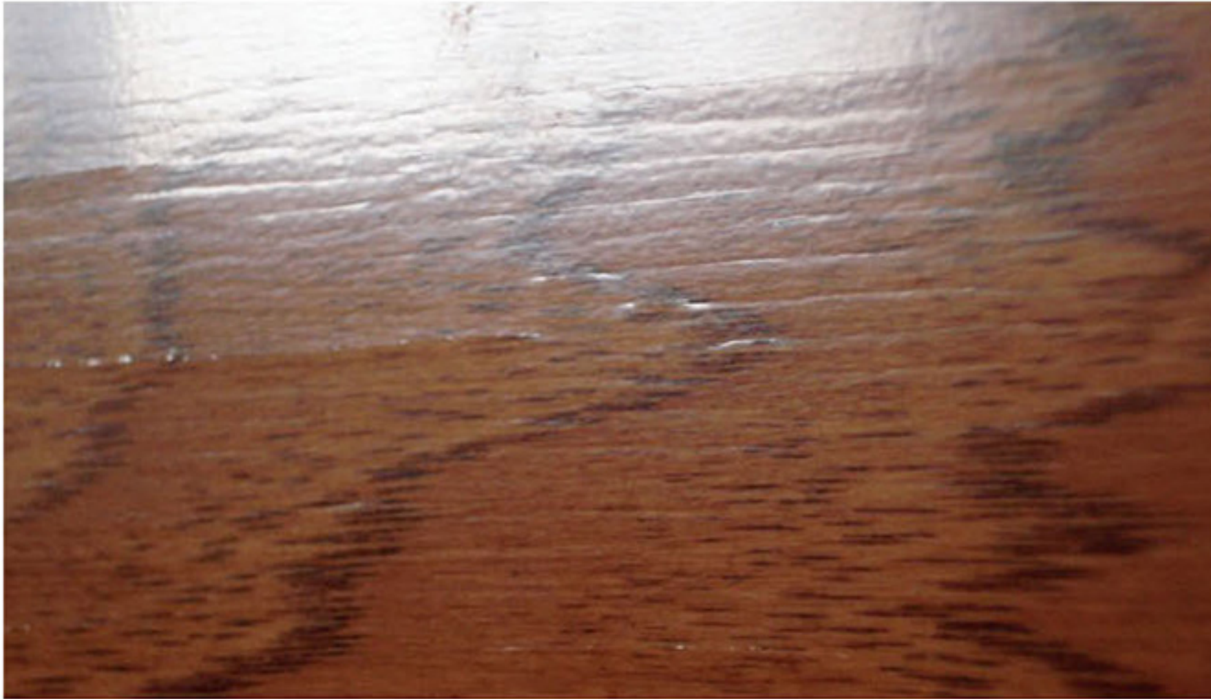
Telescoping lathe checks on rotary-peeled lamella
